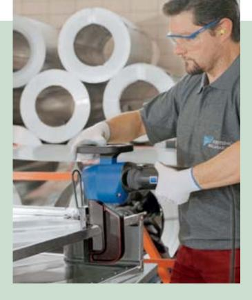
Whether in HVAC or in container and equipment construction, joining is probably the simplest and most cost-effective way to connect two metal parts. The TRUMPF power fastener uses a unique cold-forming technology to punch a small dimple into both sheets— and immediately you have an astonishingly stable, long-lasting connection. No screws, no rivets, no emissions, no preparation or cleanup work.
